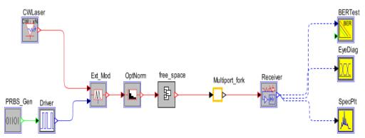
Figure.3. Simulation setup for FSO link
