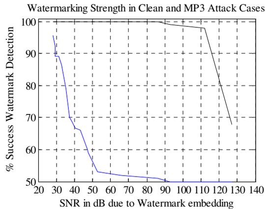
Figure 6. Effect of watermark embedding strength in clean and MP3 attack. **Blue:** MP3 attack. **Black:** No Attack
