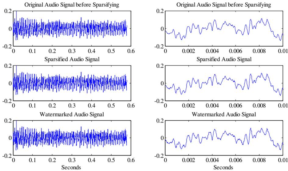
Figure 2. Original, sparsified and watermarked segments. Left: 0.6 sec. segment. Right: 0.01 sec. segment.
