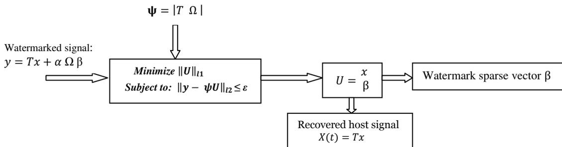
Figure 3. Diagram of the Watermark Recovery Process
