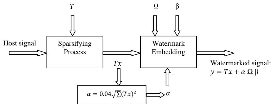
Figure 1. Diagram of the Watermark Embedding Process
