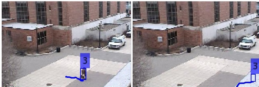
Fig. 7. Test case of object occluded by a roof (occlusion due to obstacle)
