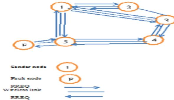
Figure 1: Black Hole Attack Specification
