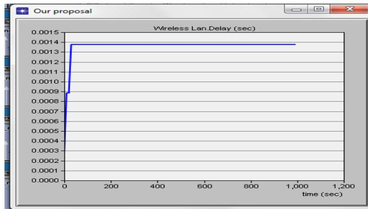
Figure 8: Delay with Apply OLSR protocol
