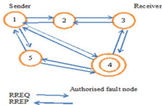
Figure2: Internal black hole attack
