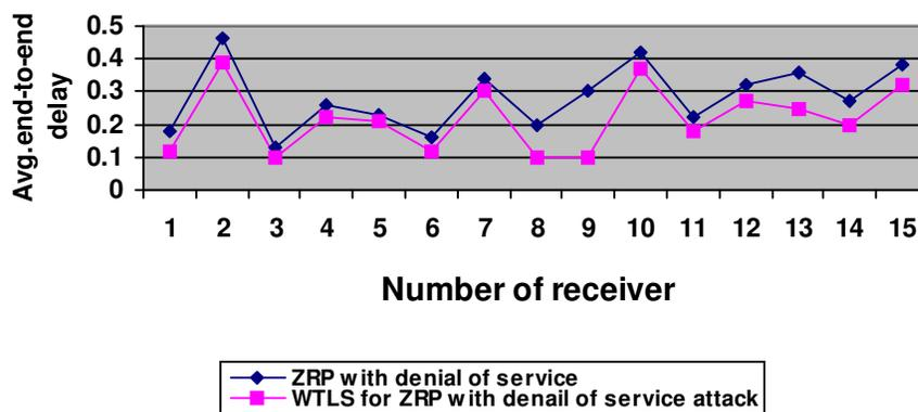
Figure 6: Comparison of End to End delay of ZRP and ZRP for WTLS with Denial of Service attack
