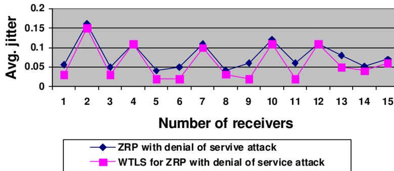
Figure 5: Comparison of Average Jitter of ZRP and ZRP for WTLS with Denial of Service attack
