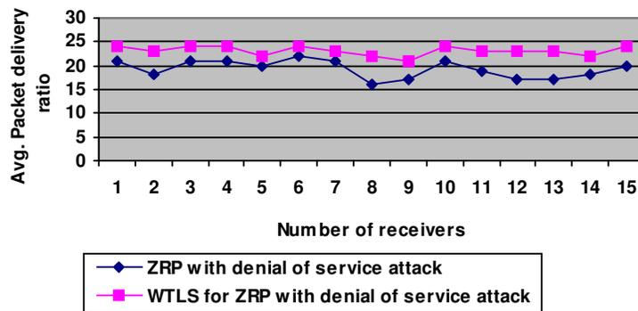
Figure 3. Comparison of Average packet delivery ratio of ZRP and ZRP for WTLS with Denial of Service attack
