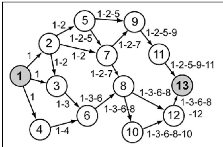
Figure 4. Building of the record during route discovery in DSR
