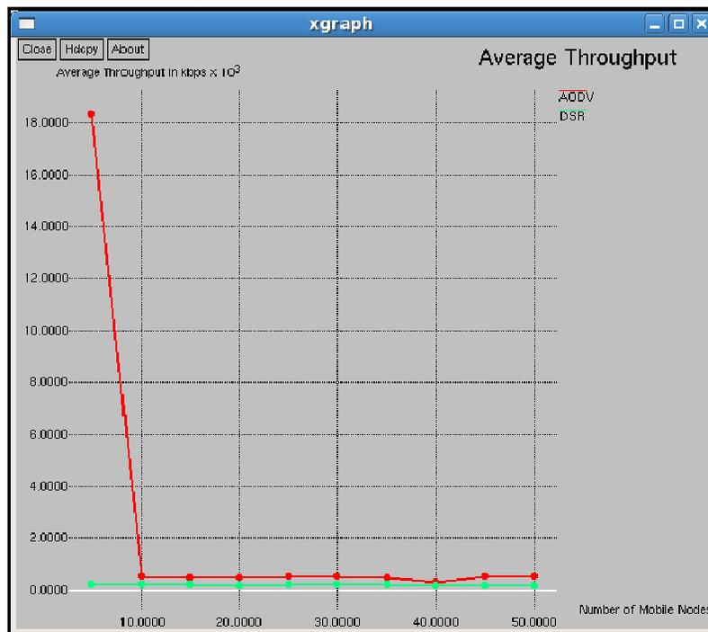
Figure 15. Throughput for AODV and DSR with varying no. of Mobile Nodes
