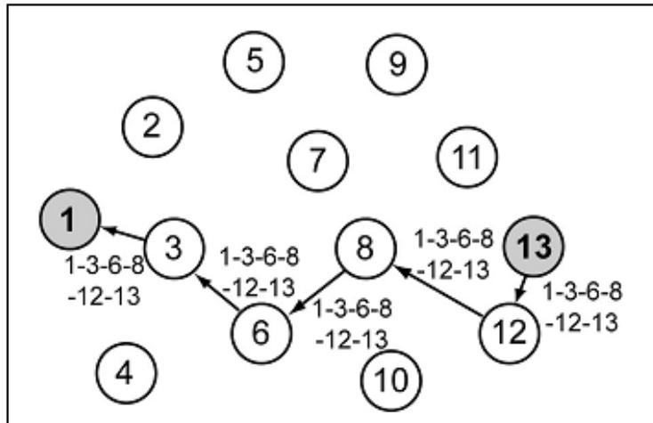
Figure 5. Propagation of the route reply in DSR
