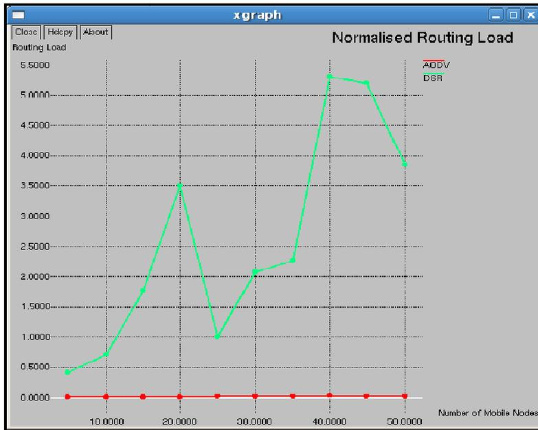
Figure 14. Normalized routing Load for AODV and DSR with varying no. of Mobile Nodes
