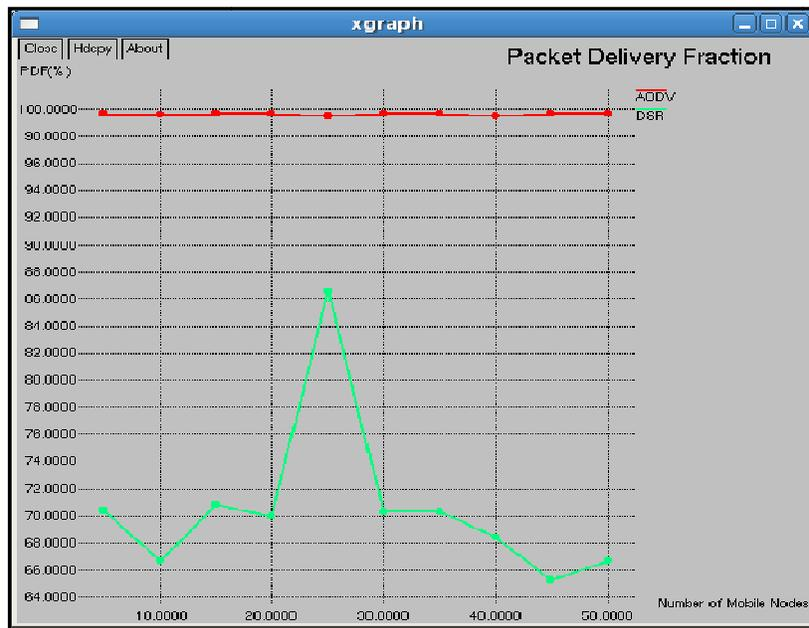
Figure 12. Packet Delivery Fraction for AODV and DSR with varying no. of Mobile Nodes
