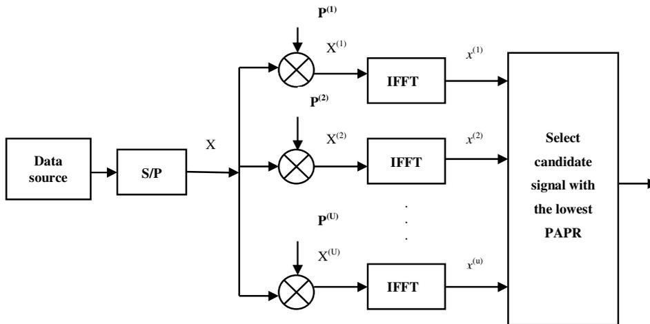
Figure 1. The block diagram of SLM scheme
