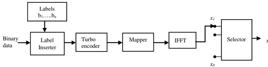
Figure 3. Turbo Coded OFDM System Model
