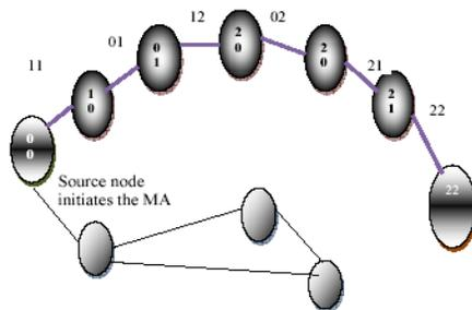
**Fig 3:** Nodes have unique ID compute by debruijn graph
