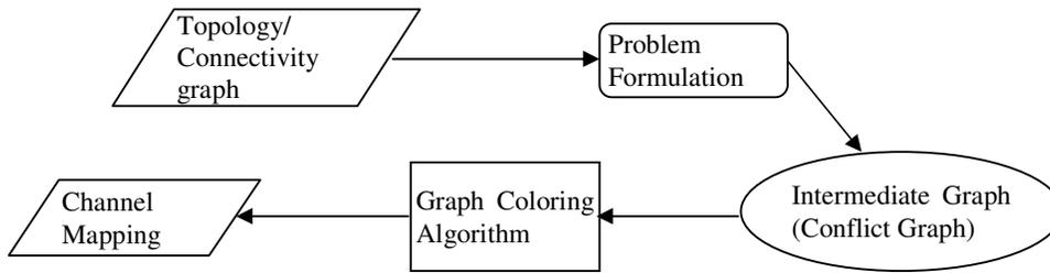
Figure 5. Framework for channel assignment
