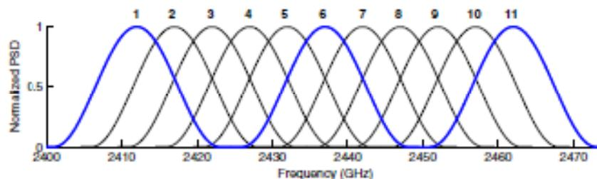
Figure 10. IEEE 802.11b/g channel distribution showing the 3 orthogonal channels in blue [65]
