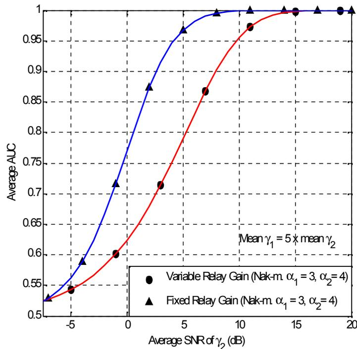
Figure 8. Comparison of variable relay gain and fixed relay gain based spectrum sensing
