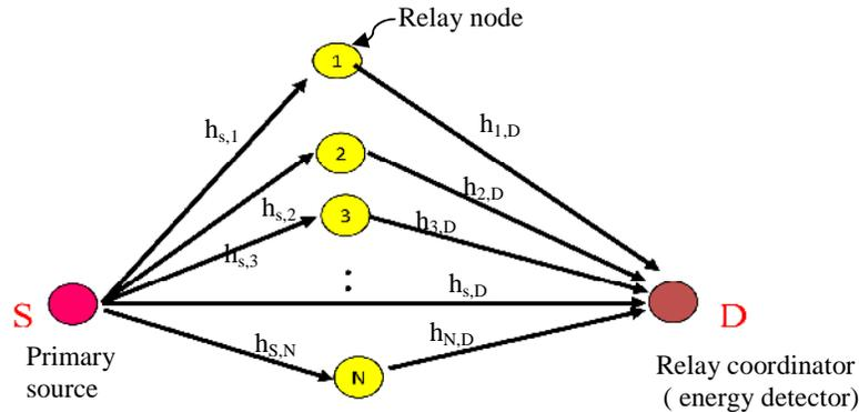
Figure 1. Relay based spectrum sensing
