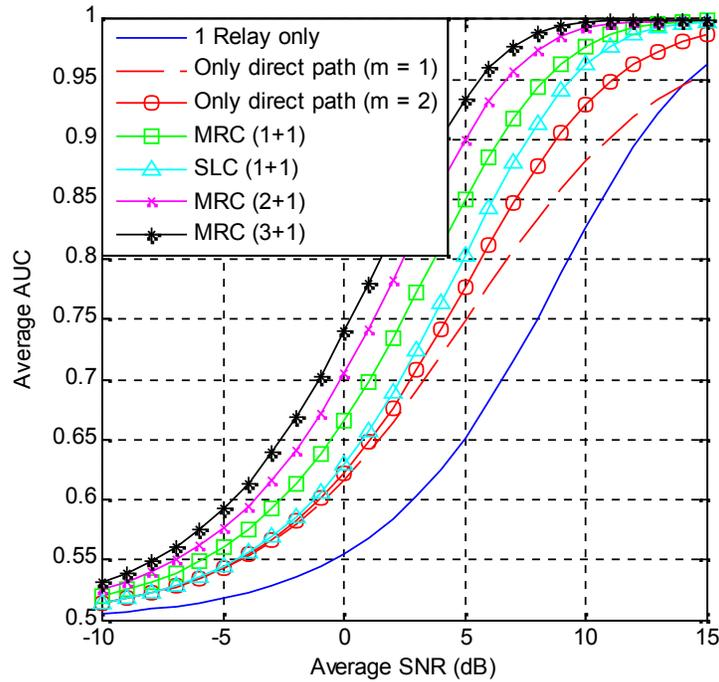
Figure 2. Average AUC vs. mean SNR for N-relay network with source to destination direct path over *i.i.d.* Nakagami- $m$  Channels ( $m = 2$  and  $u = 3.5$ ).
