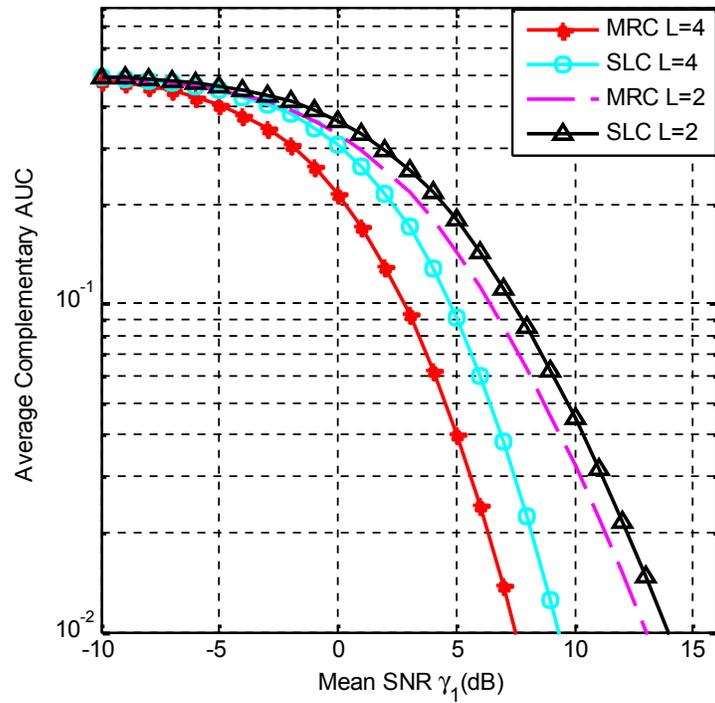
Figure 6. Complementary AUC. Comparison of MRC with SLC diversity combining schemes for a fixed AF dual-hop relay network over Rayleigh fading ( $u = 2, \bar{\gamma}_2 = 5\bar{\gamma}_1$ ).
