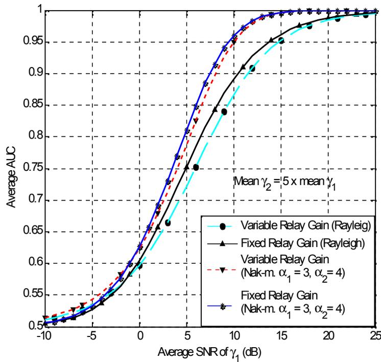
Figure 7. Fixed and variable relay gain performance over fading channels using unified SNR model with  $u = 2$ .
