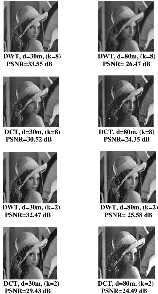
Figure 5. Obtained images with different distance for Lena 64x64
