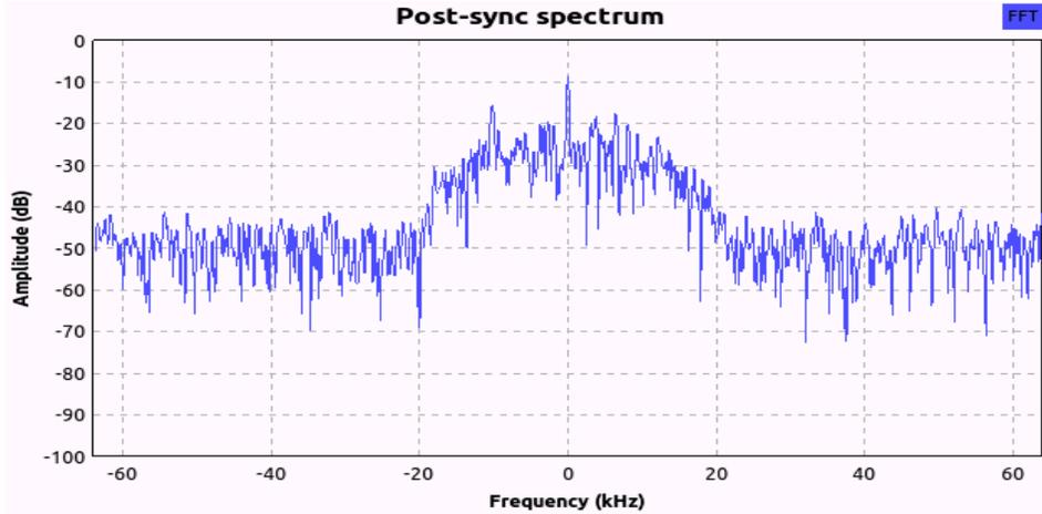
Figure 8: Post synchronized spectrum with effect of channel noise is 100m units.
