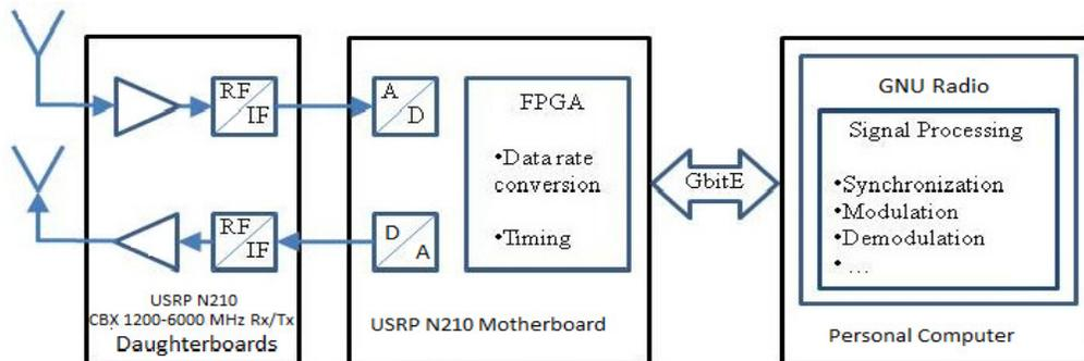
Figure 1: Software Defined Radio block diagram with USRP N210 and GNU Radio.
