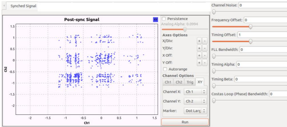
Figure 7: Post synchronized spectrum without channel effect.
