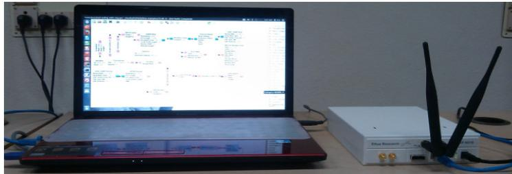
Figure 3: Software Defined Radio development test bed.
