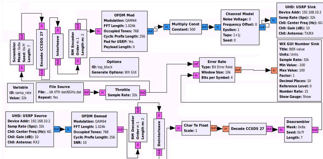
Figure 4: GNU Schematic for OFDM transmission and reception over USRP source and sink for BER analysis.
