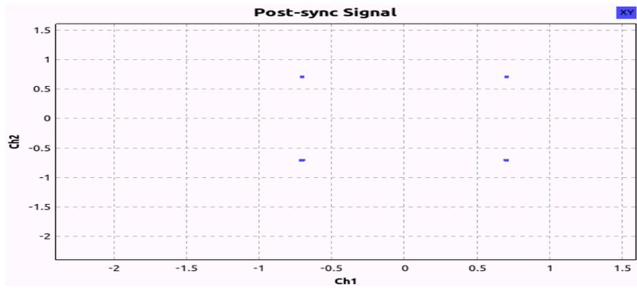
Figure 12: Post synchronized signal with effect of timing alpha is 20m units.
