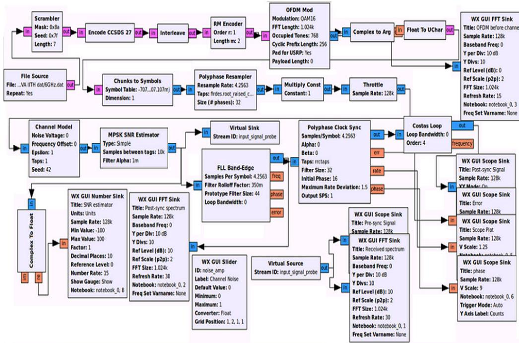
Figure 2: GNU schematic for OFDM signal transmission and reception over virtual source and sink.
