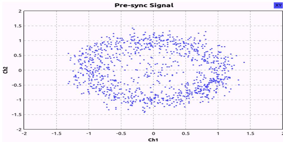
Figure 10: Received signal with effect of frequency offset is 11m units.
