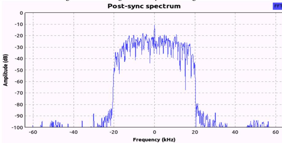
Figure 6: Post synchronized spectrum without channel effect.
