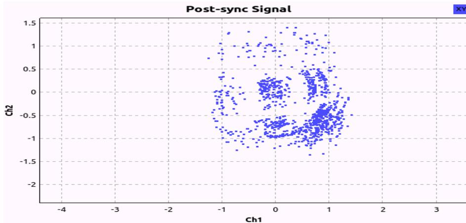
Figure 13: Post synchronized signal with effect of Costas loop (phase) bandwidth is 10m units.
