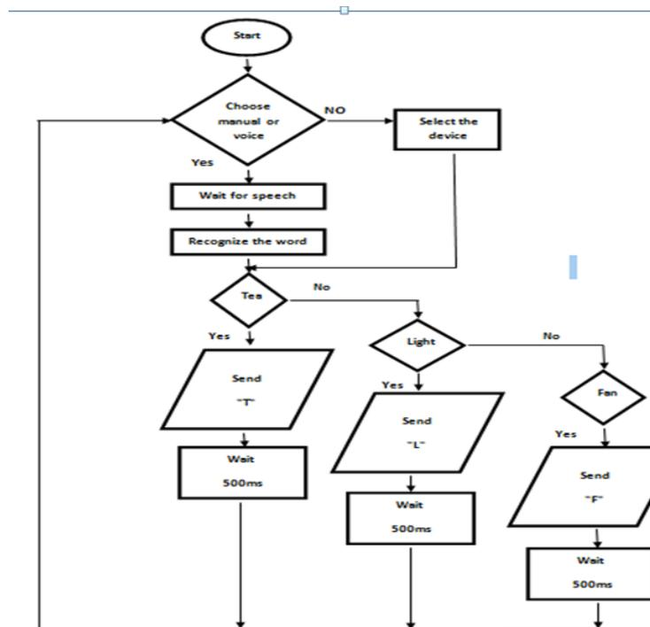
Figure 5 The flowchart for the operation of the transmitter.
