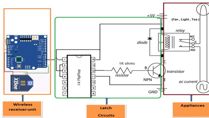
Figure 7. The latch circuit
