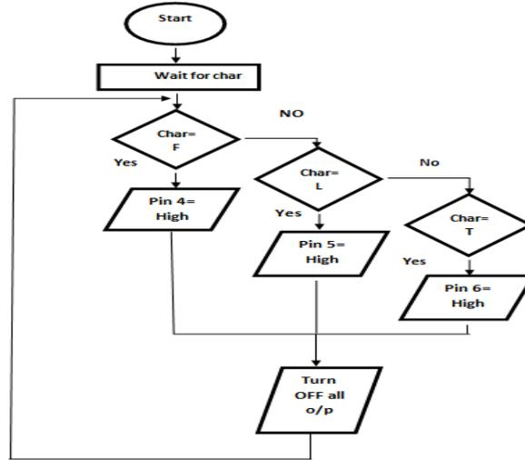
Figure 6 The flowchart for the operation of the receiver
