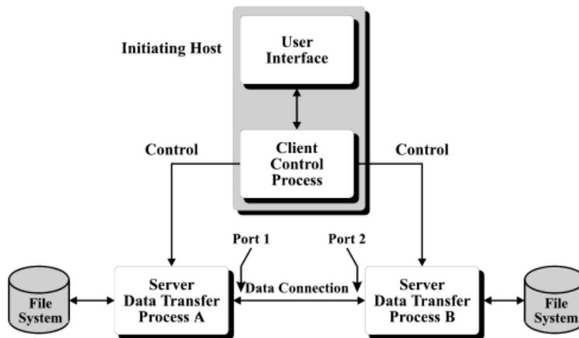
Figure 10. FTP Client Server Process
