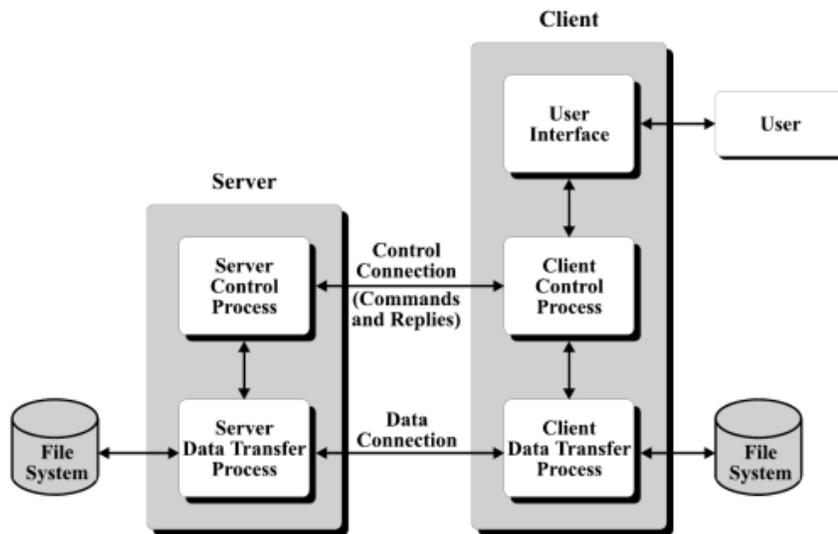
Figure 9. FTP Client-Server Application
