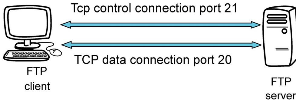
Figure 7. Control and data connection
