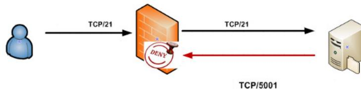
Figure 11. Active FTP and Firewall
