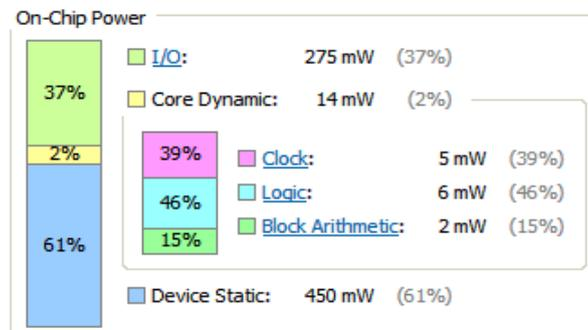
Figure 28. Power Estimation of Transmitter
