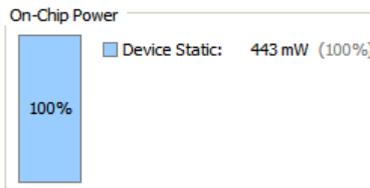
Figure 27. Power Estimation of Receiver
