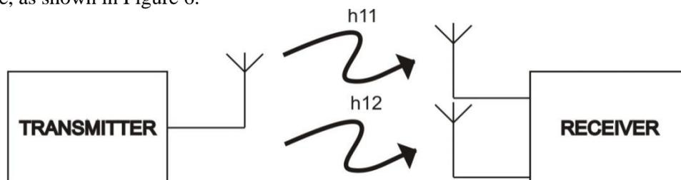
Figure 6. Basic block diagram of SIMO
