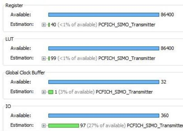
Figure 22. Resource Estimation of Transmitter
