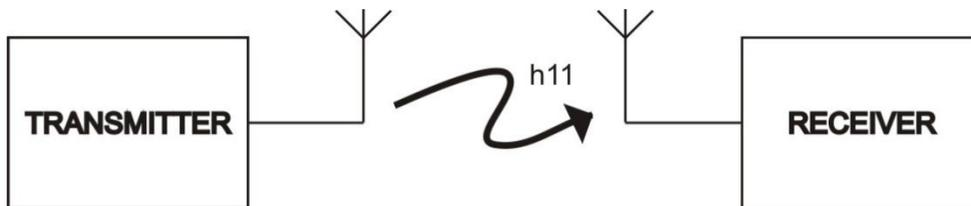
Figure 2. Basic block diagram of SISO
