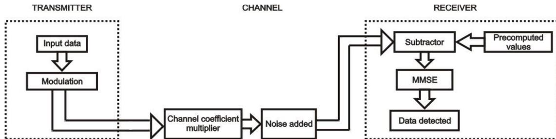
Figure 1. System Model of Channel Emulation process
