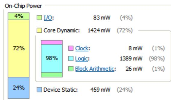
Figure 30. Power Estimation of Receiver
