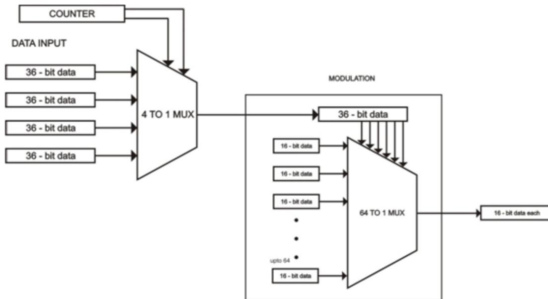
Figure 3. Transmitter side architecture of SISO
