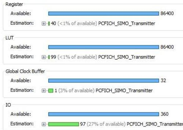
Figure 19. Resource Estimation of Transmitter
