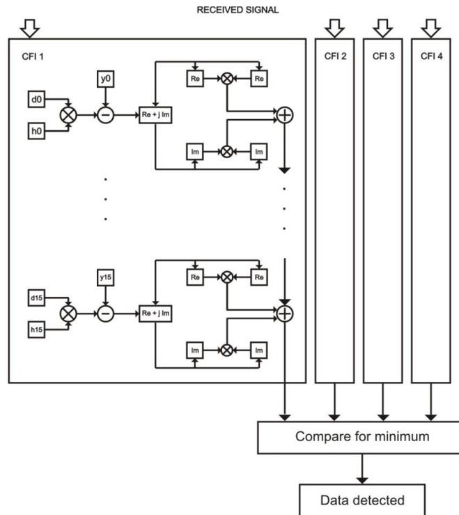
Figure 5. Receiver side architecture of SISO
