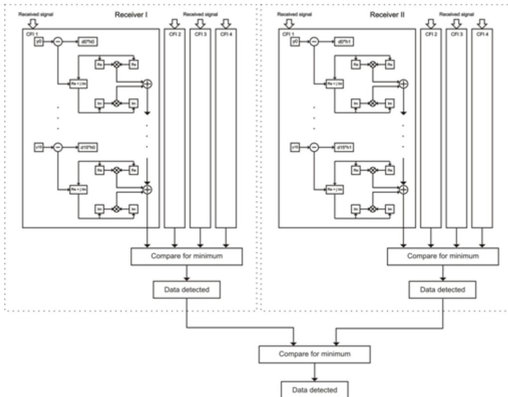
Figure 8. Receiver side architecture of SIMO
