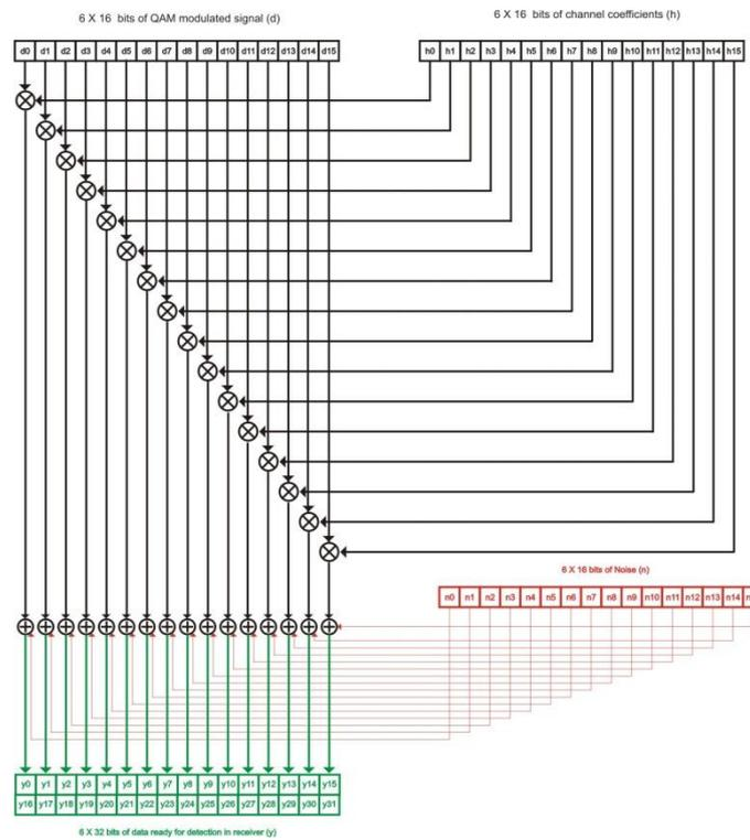
Figure 4. Channel Estimation architecture of SISO
