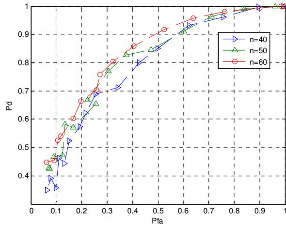
Figure 6. ROC curve for ED method with  $m=8$  and  $SNR=10dB$
