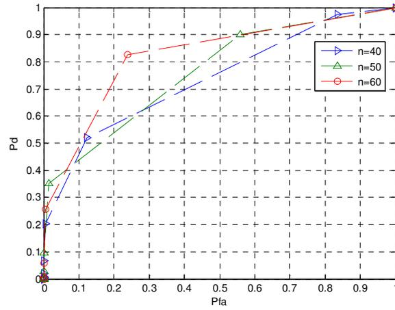
Figure 7. ROC curve for GLRT method with  $m=8$  and  $SNR=10dB$
