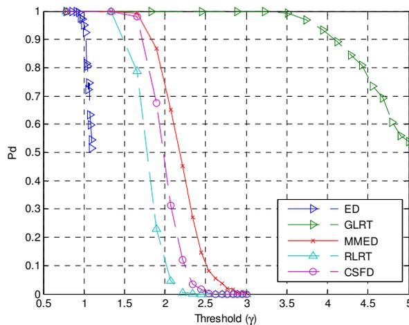
Figure 11.  $P_d$  Vs Threshold for all sensing methods
