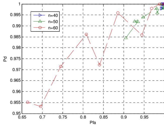
Figure 9. ROC curve for MMED method with  $m=8$  and  $SNR=10dB$
