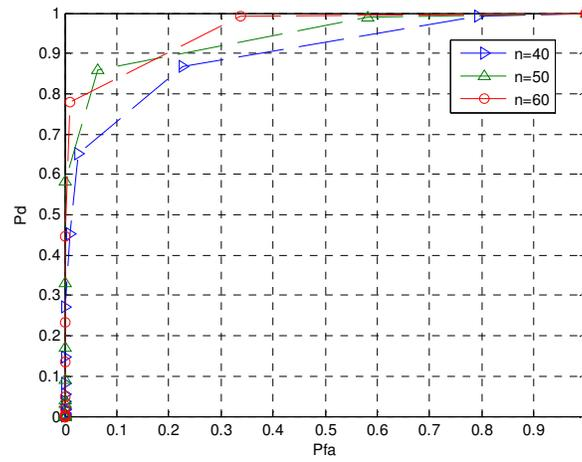
Figure 8. ROC curve for CSFD method with  $m=8$  and  $SNR=10dB$
