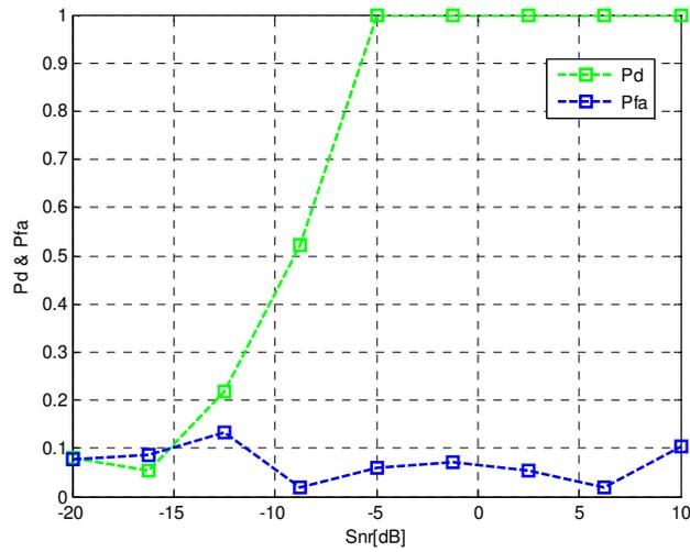
Figure 5. Pd, Pfa Vs SNR
