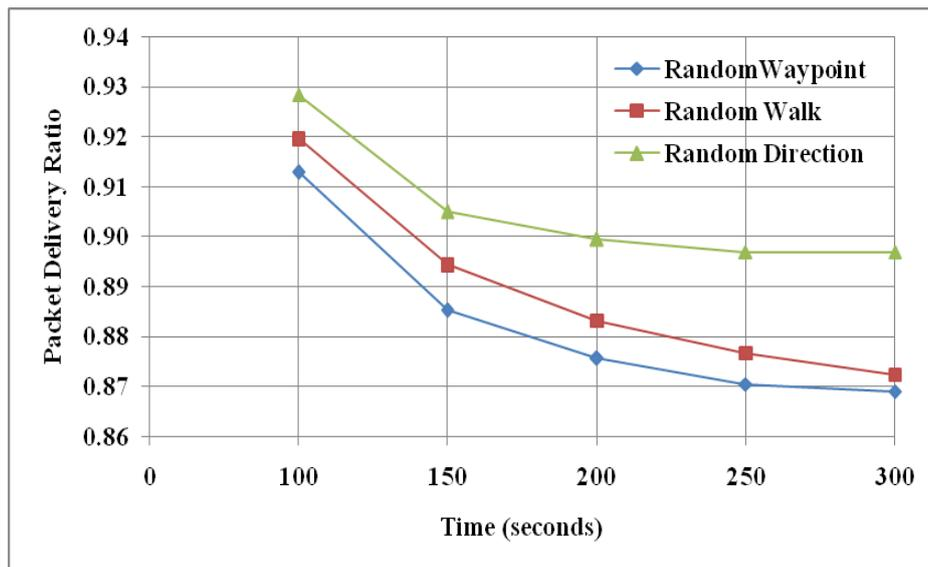
Figure 7. Packet Delivery Ratio in OLSR using three mobility models over simulation time
