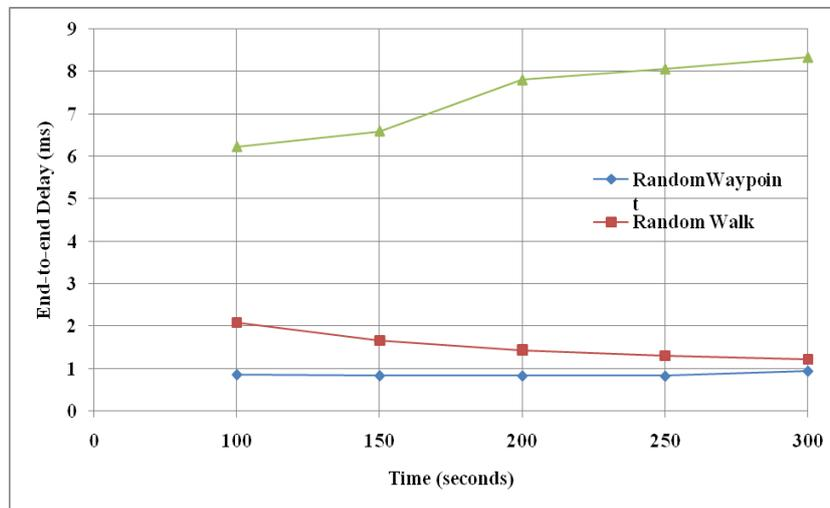
Figure 6. End-to-end Delay in OLSR using three mobility models over simulation time
