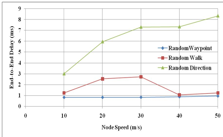
Figure 3. End-to-end delay in OLSR using three mobility models over varying speed
