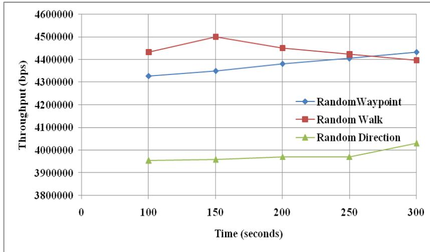
Figure 5. Throughput of OLSR using three mobility models over simulation time
