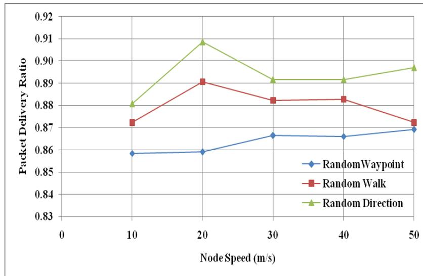
Figure 4. Packet Delivery Ratio in OLSR using three mobility models over varying speed
