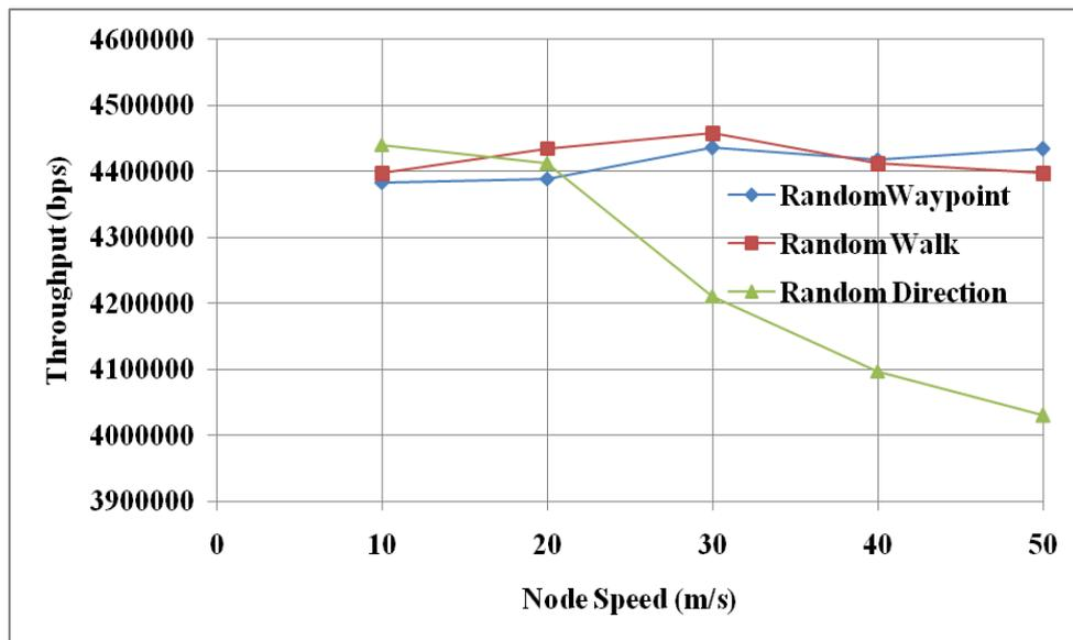
Figure 2. Throughput of OLSR using three mobility models over varying speed
