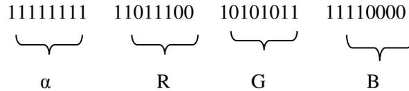
Figure 1.1 Bit Representation of a 32-bit RGB Pixel
