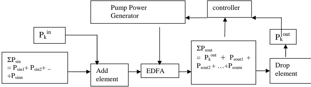
Figure 8: Security envelope for attack monitoring and on-the-fly gain restoration during attack
