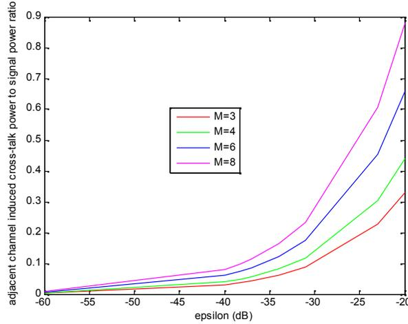
Figure 11: The ratio of worst case  $\lambda_{21}$  induced crosstalk power to the signal power in  $\lambda_{11}$  versus component crosstalk
