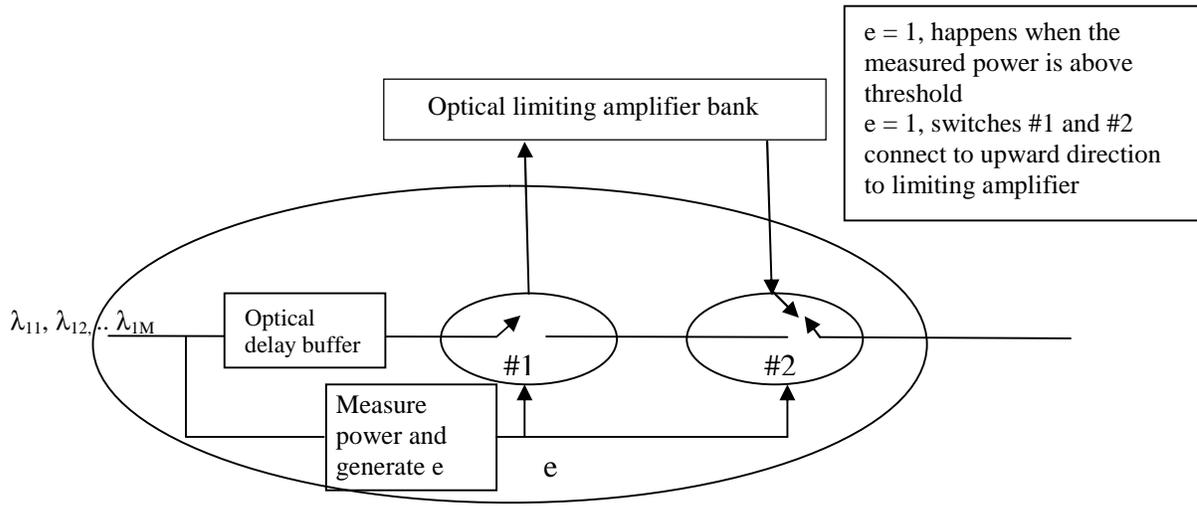
Figure 14: Detouring of light path via power limiters when measured fiber power is high
