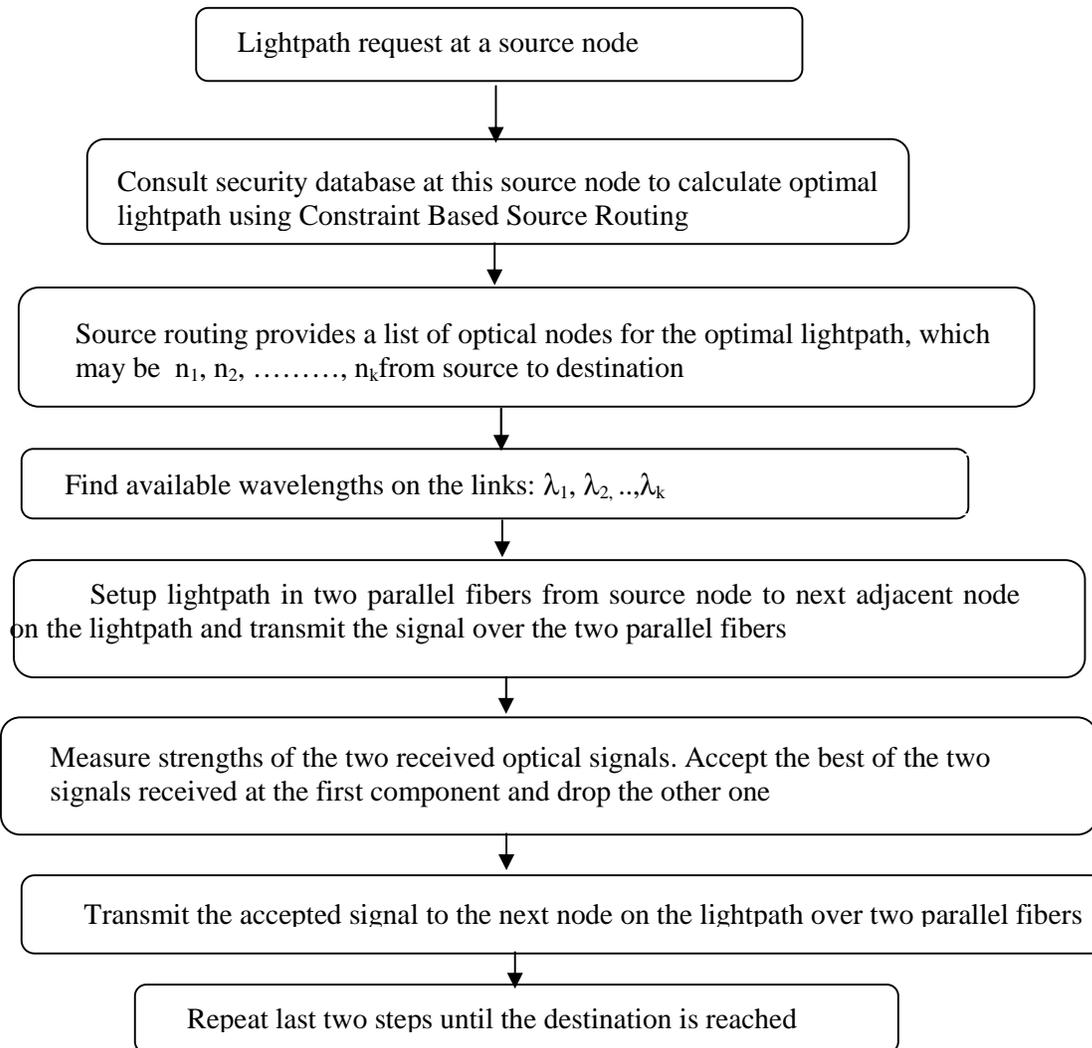
Figure 5: Fiber diversity based data transmission in secure lightpath
