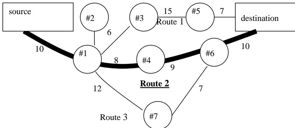
Figure 4: Calculation of secured lightpath from a source to a destination in an example network
