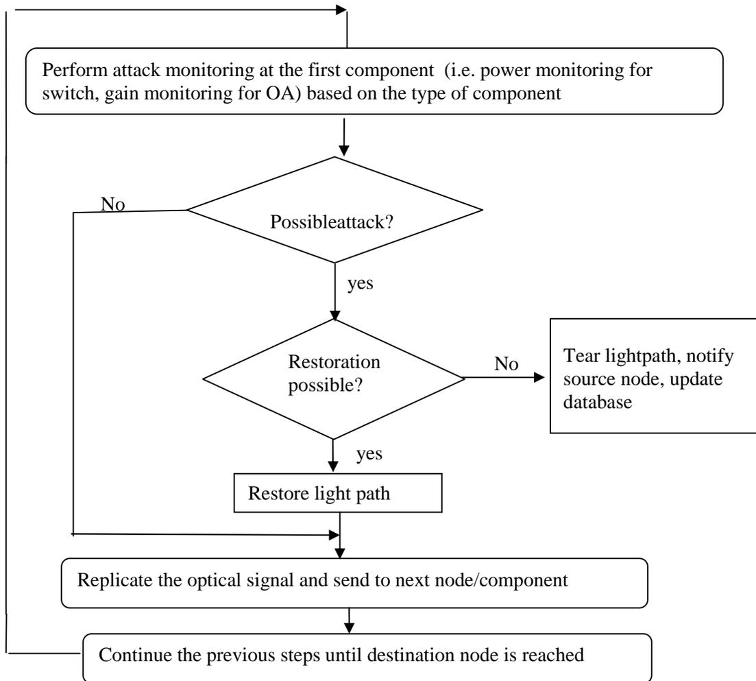
Figure 6. Attack monitoring and restoration in the components in light path
