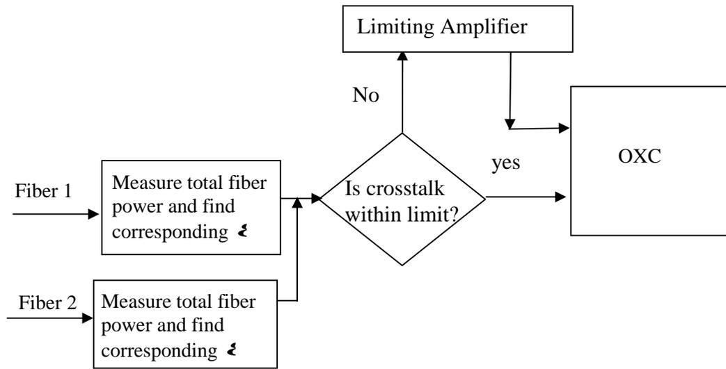
Figure 12. Outline of monitoring and restoration of out of range crosstalk in switches
