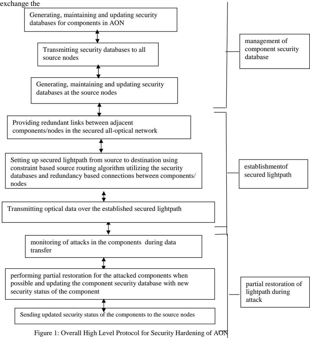
Figure 1: Overall High Level Protocol for Security Hardening of AON
