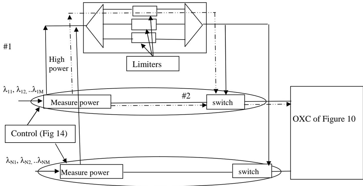
Fig 13: Proposed security envelope to control the high power jamming attack
