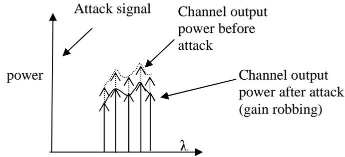
Figure 7: EDFA attack and gain robbing
