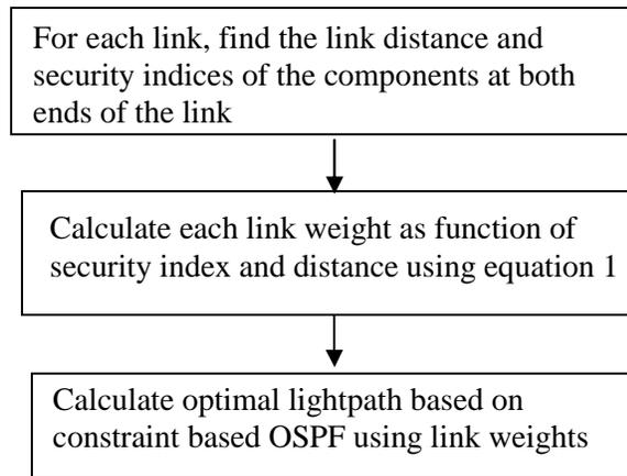
Figure 3: Flow chart of constraint based source routing to select optimal lightpath
