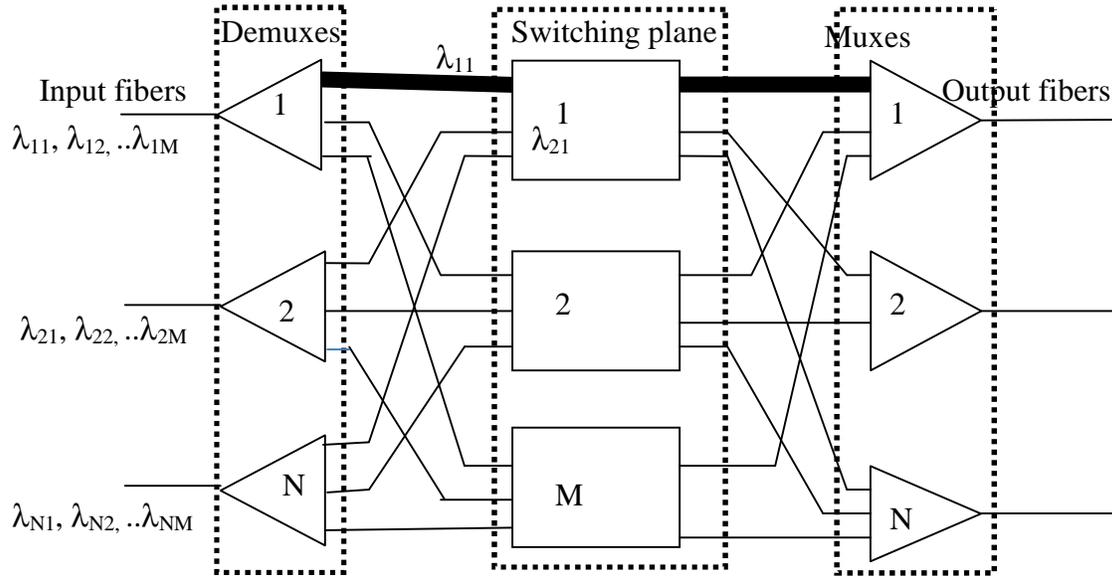
Figure10: A typical N\*M OXC over which the crosstalk characteristics have been studied
