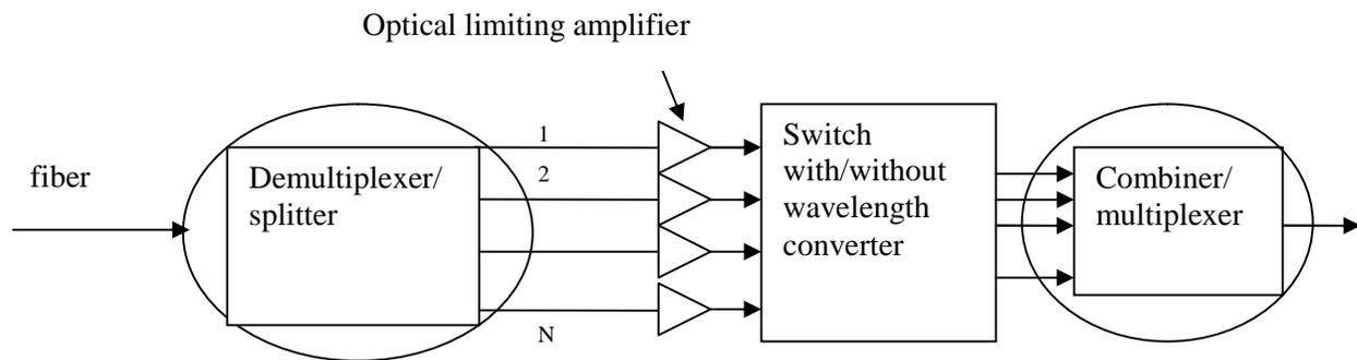
Figure 9: incorporating pre-emphasis/de-emphasis filter within an OXC of AON
