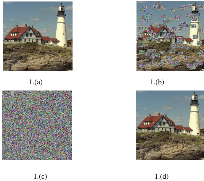
Figure1.(a)Original Image, 1.(b) Hash attached Partially Encrypted image, 1.(c) Permutation With Partially Encrypted Hash Attached Image, 1.(d) Decrypted Image
