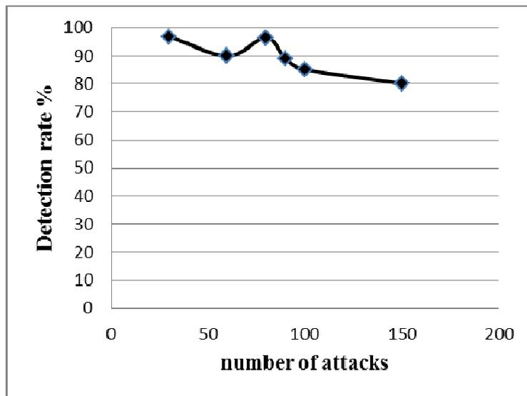
Figure 7 Effect of number of hello flood attack on detection rate
